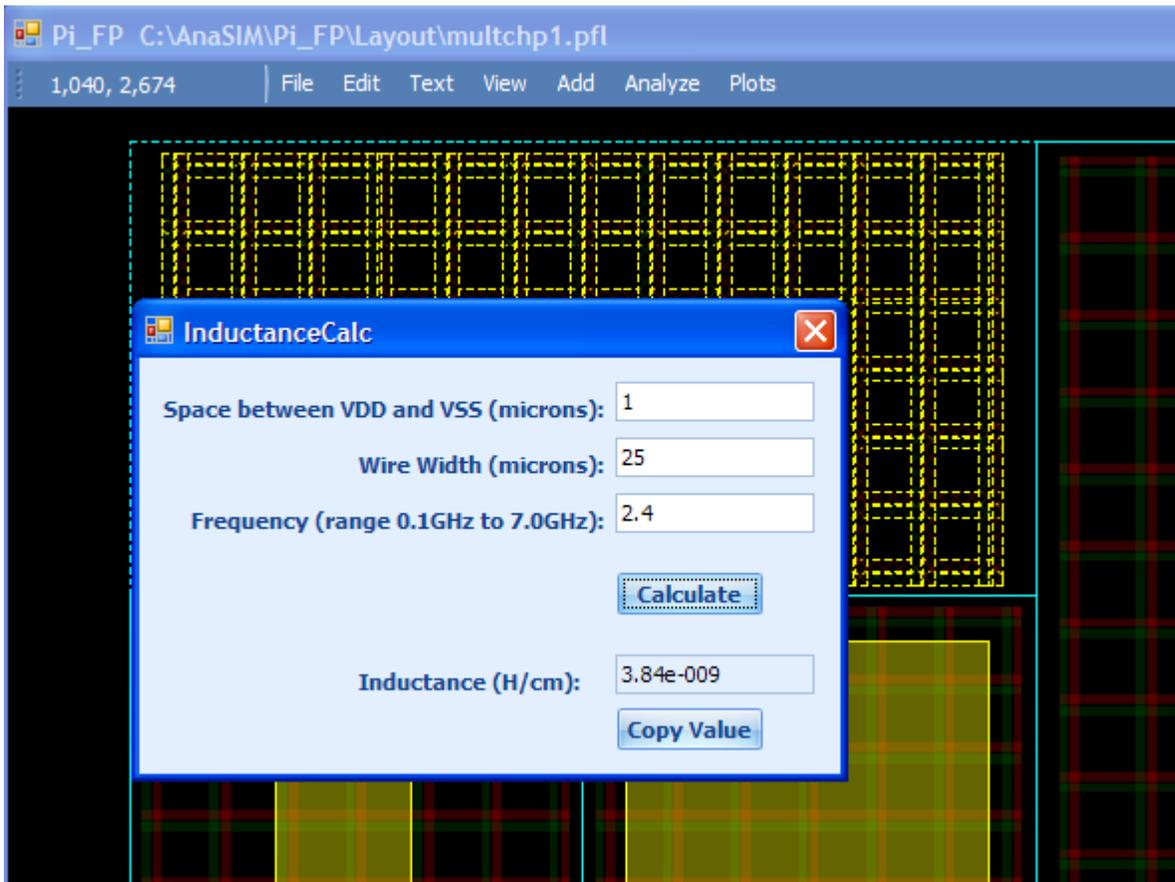
Figure 2:  $\pi$ -fp power grid inductance calculation
