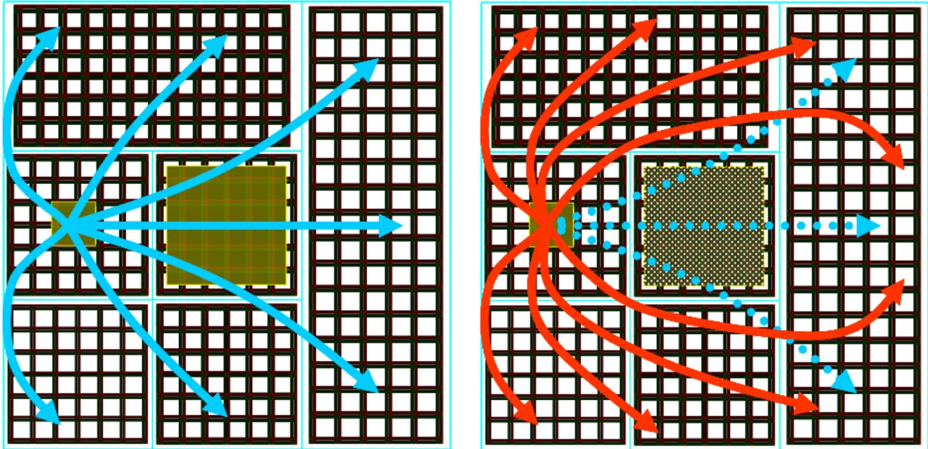
**Figure 4: Noise propagation without and with power gating**
