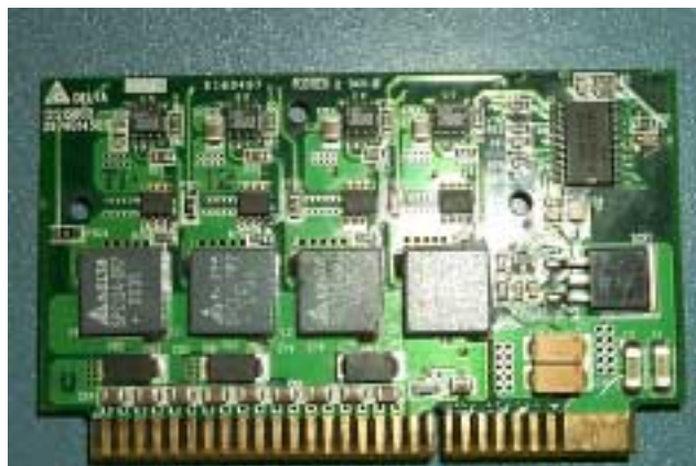
Figure 3: A Voltage Regulator Module (VRM)
