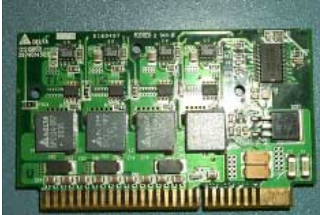
Figure 3: A Voltage Regulator Module (VRM)
